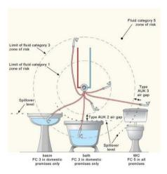
Robust factory applied retaining rings of the design which do not allow the shower hose to be removed are a recognised method of maintaining an AUK3 air gap acceptable in all types of premises. For further information please refer to <u>www.waterregs.couk/guidance</u> information note <u>'Prevention of the risk of backflow in the design of domestic bathrooms'.</u>
